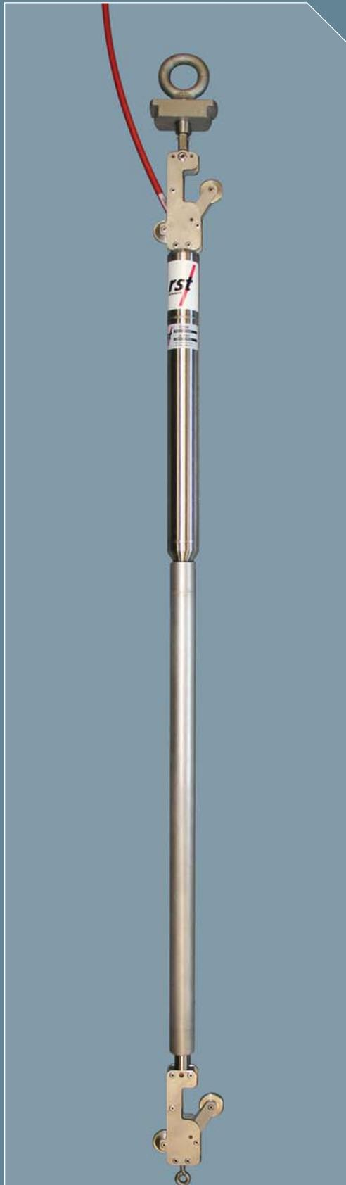
Vertical In-place MEMS Inclinometer Systems are designed to measure lateral movement of soil and rock or deflection of man made structures such as piles or retaining walls, when remote and continuous monitoring is required.
