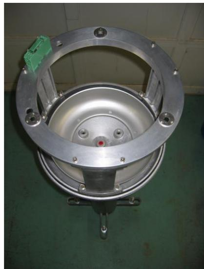
(Photo 2-3 – Gauge frame on Pedestal)
