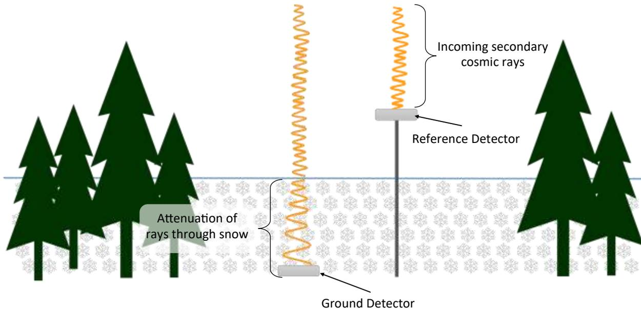
A ground detector is installed flush with the soil and a reference detector is installed above the maximum snow height. The reference detector will correct for any moisture that is attenuated through the atmosphere as well as allow for change over space in the natural variation of incoming cosmic radiation.
