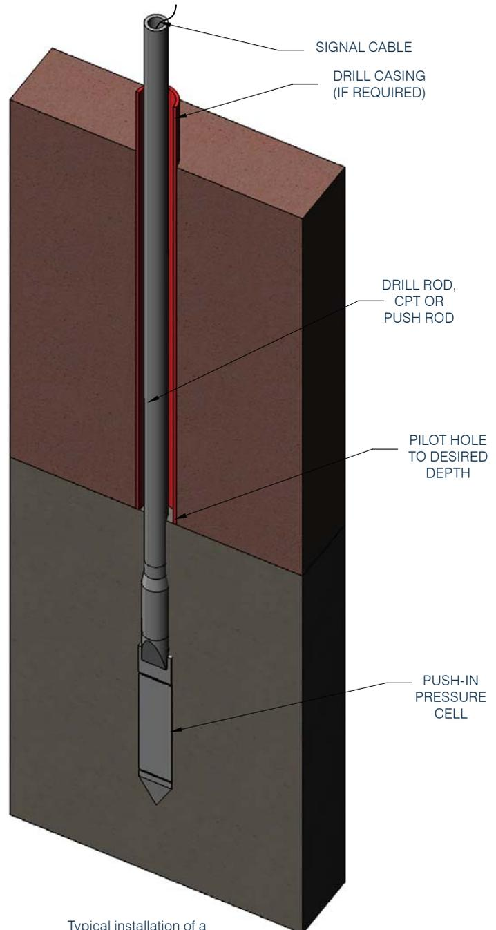
Typical installation of a
