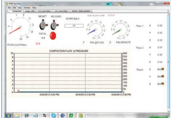
Screenshot of Real-time Monitoring Software showing grouting parameters in real-time.
